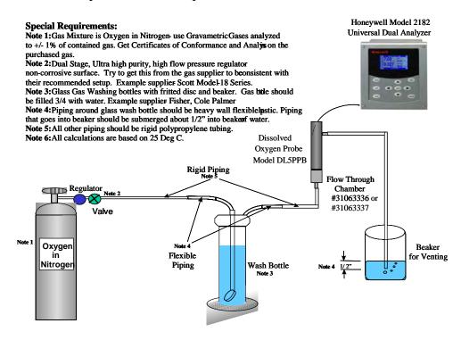
Figure 15-7 Suggested ppb Dissolved Oxygen Test Set-up
